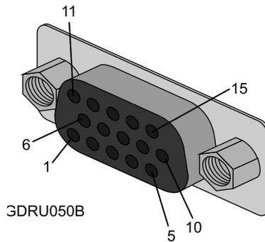
**15-Pin D-Type High Density Female Connector
