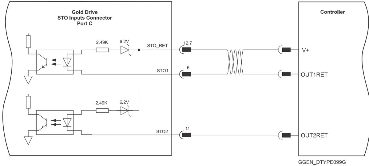
Figure 26: STO D-Type Input Connection – Sink Option
