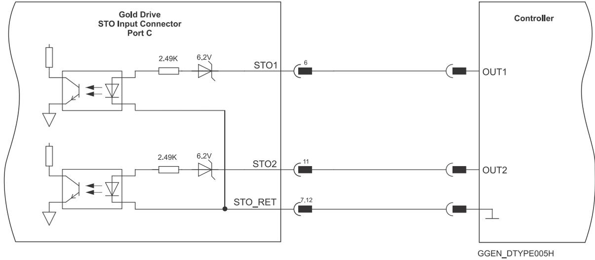
Figure 24: STO D-Type Input Connection – PLC Source Option
