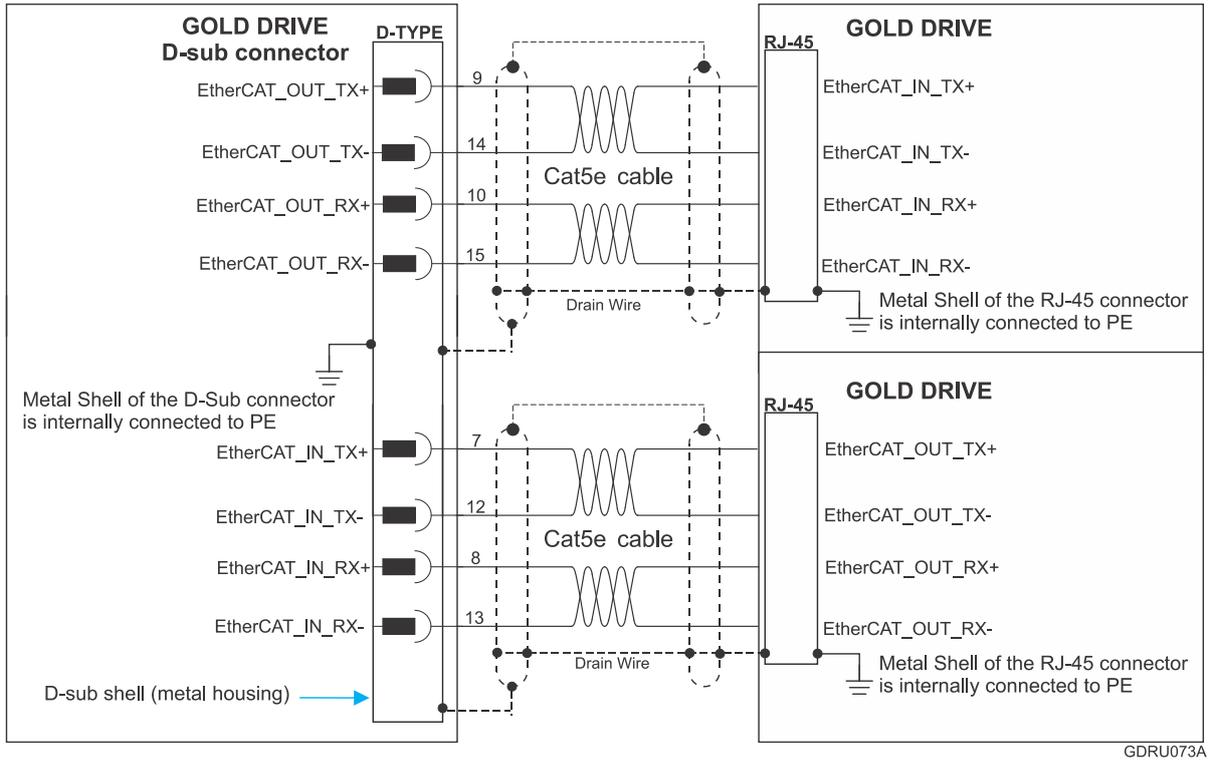
Figure 35: EtherCAT with D-Type Connections
