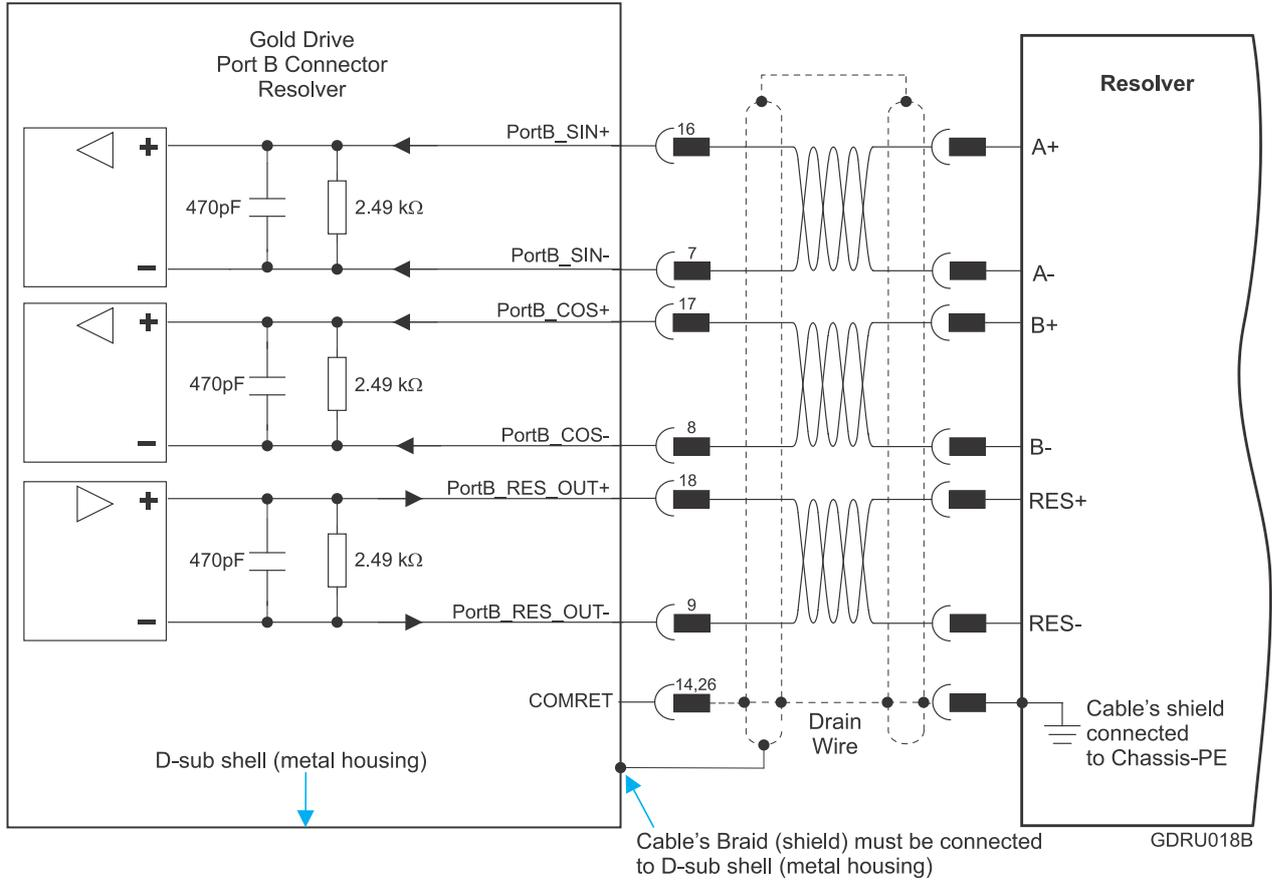
Figure 21: Port B – Resolver D-Type Connection Diagram
