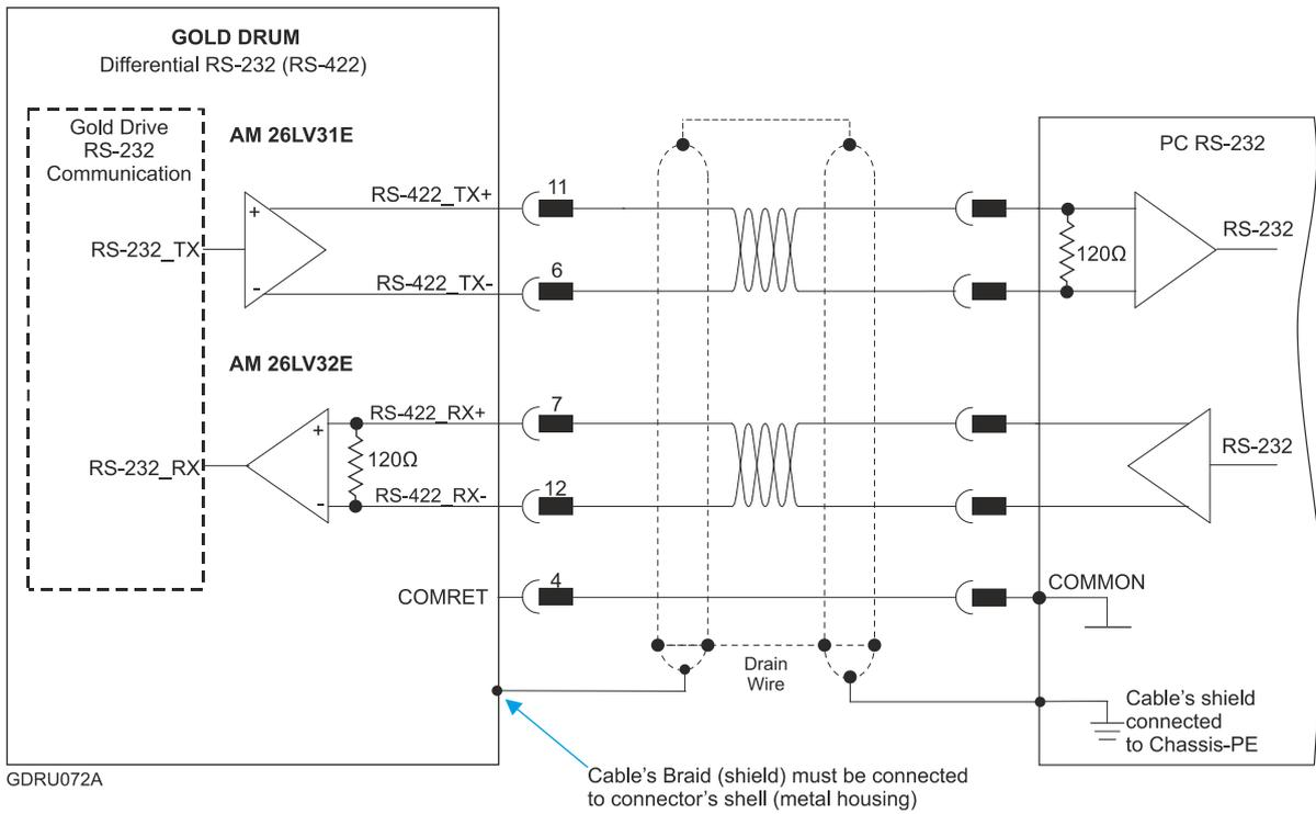
Figure 40: RS-422 (Differential RS-232) Communication Connection Diagram
