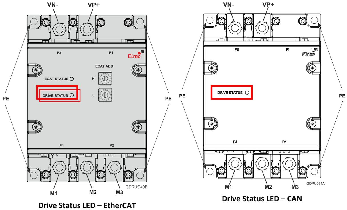
Figure 14: Drive Status LEDs
