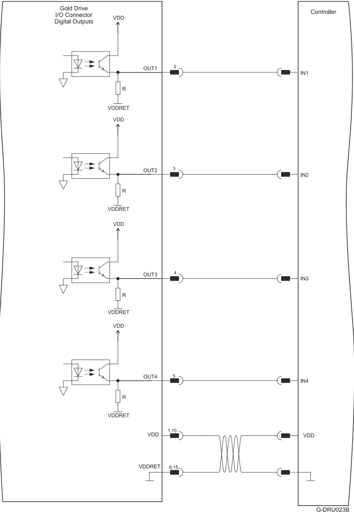
Figure 29: Digital Output D-Type Connection Diagram – TTL Option
