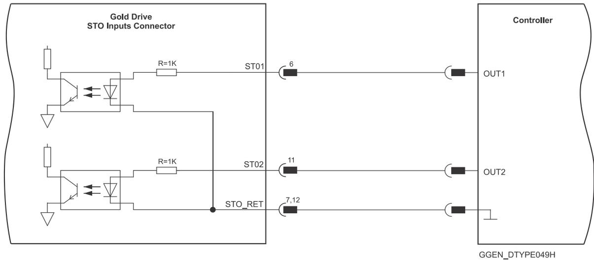
Figure 25: STO Input Connection – TTL Option
