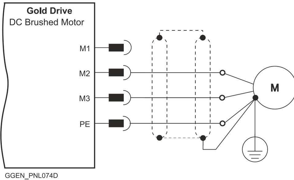
**Figure 4: DC Brushed Motor Power Connection Diagram**
