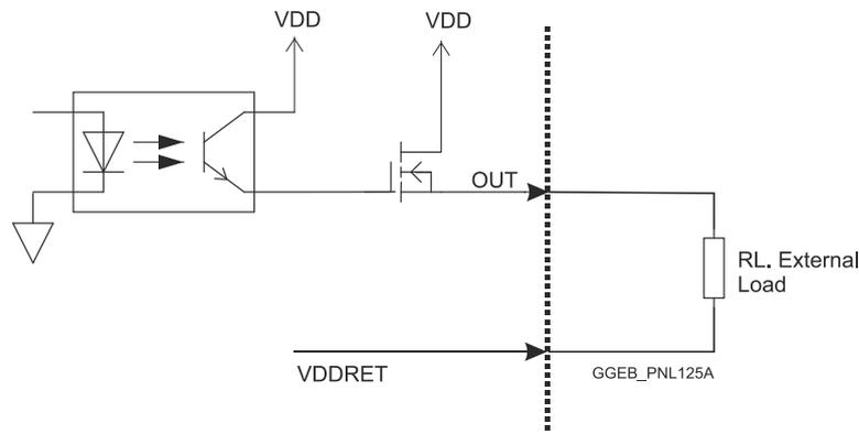
Figure 48: Digital Output Schematic – Source Mode PLC Level
