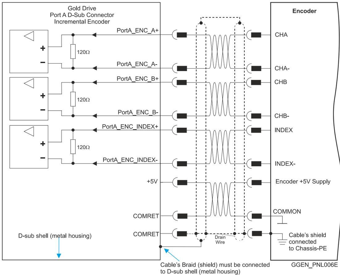
Figure 18: Port A Incremental Encoder Input – D-Type Connection Diagram Example
