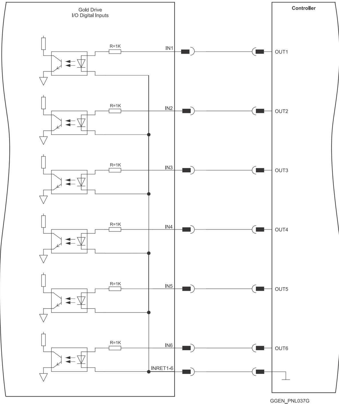
Figure 43: Digital Input TTL Mode Connection Diagram Example
