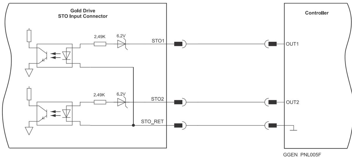
**Figure 8: STO Input Connection Example – PLC Source Option**
