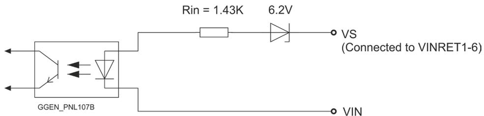
Figure 50: Digital Input Sink Schematic
