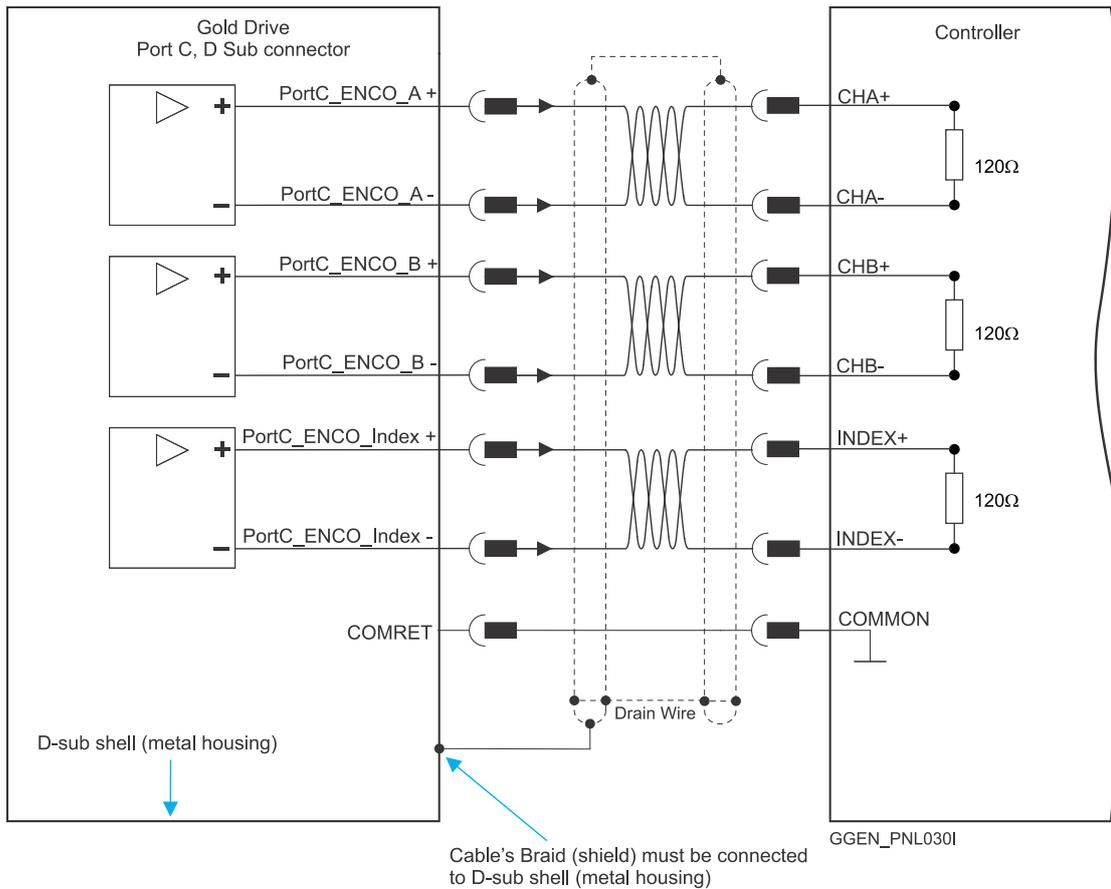
Figure 35: Encoder Differential Output – D-Type Connection Diagram Example
