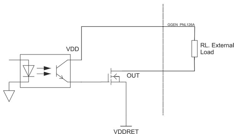
Figure 52: Digital Output Schematic for Sink – PLC level
