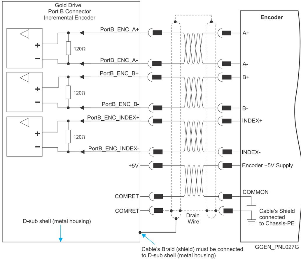
Figure 29: Port B Incremental Encoder Input – D-Type Connection Diagram Example
