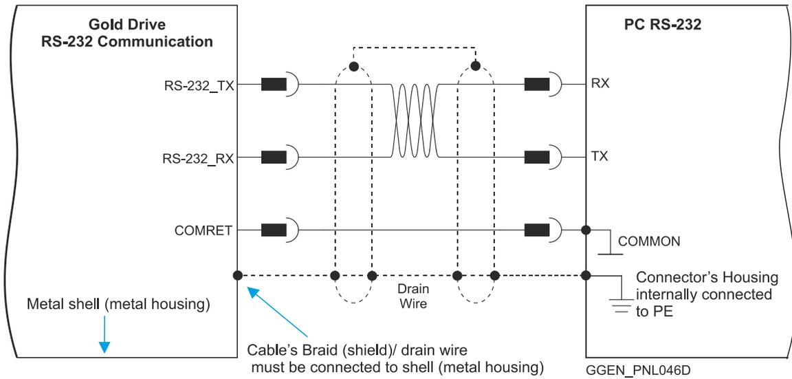
Figure 64: RS-232 D-Type Connection Diagram Example
