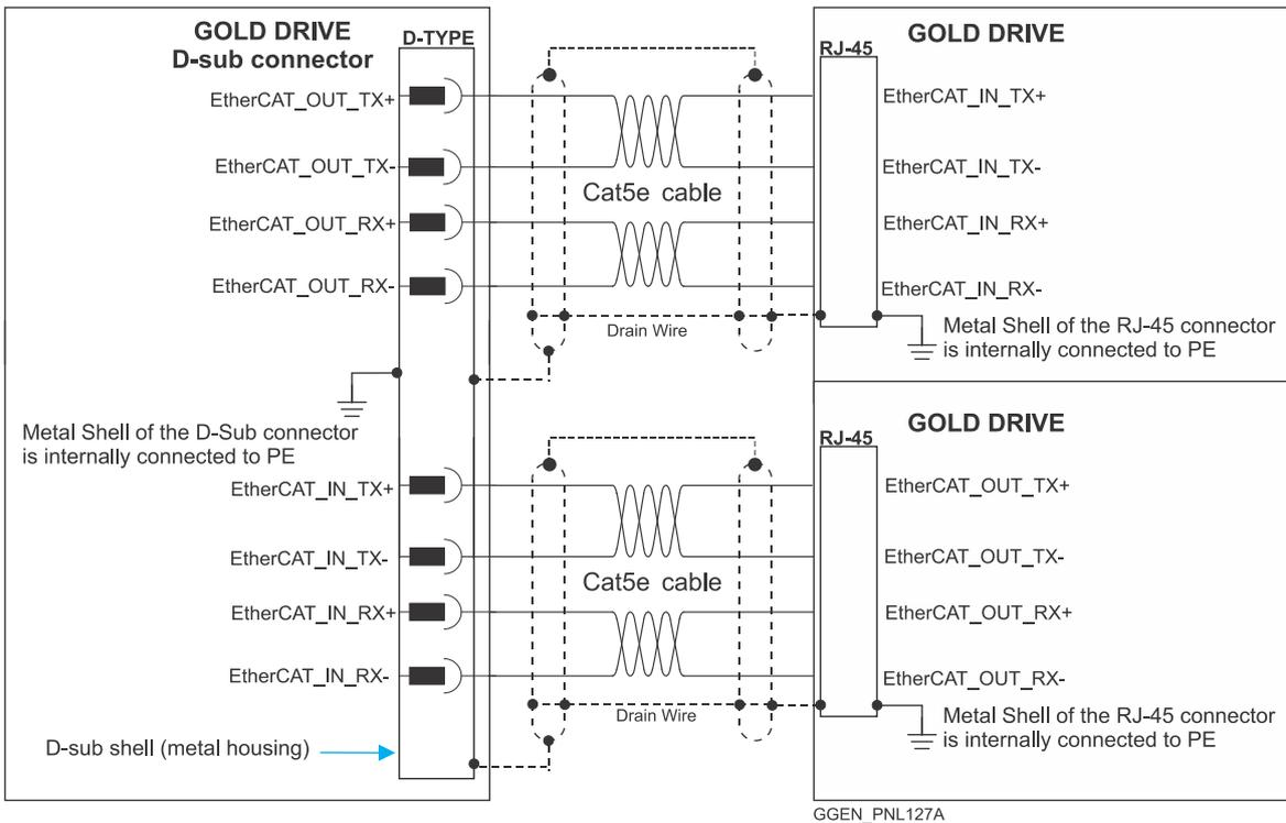
Figure 59: EtherCAT with D-TYPE Connections Example
