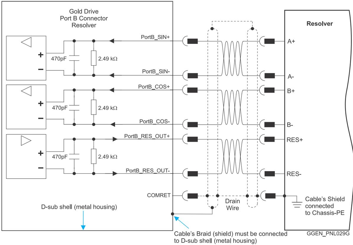
Figure 33: Port B – Resolver D-Type Connection Diagram Example
