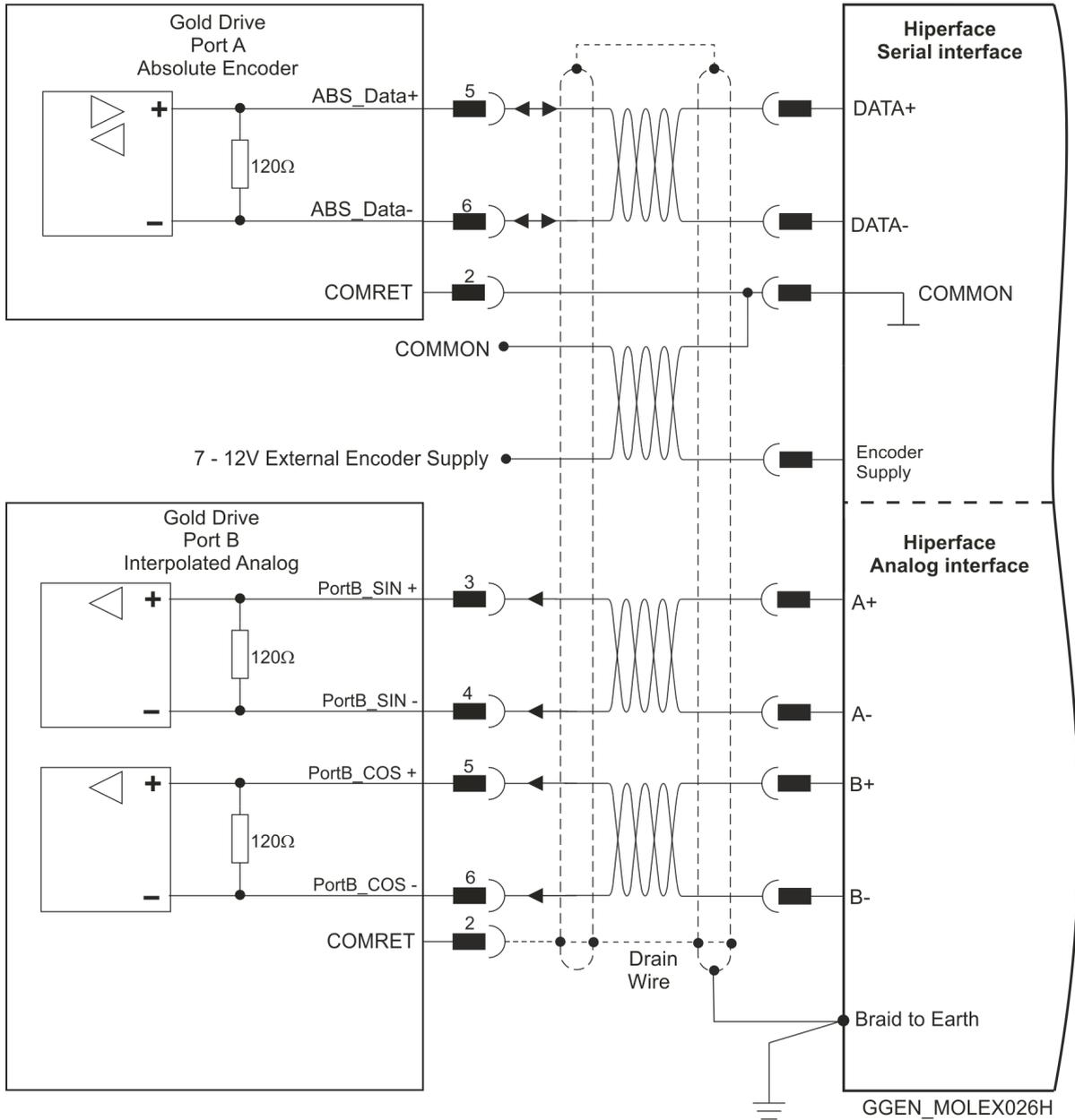
**Figure 27: Absolute Serial Encoder – Shrouded Type Connection Diagram Example for Stegmann Hiperface**
