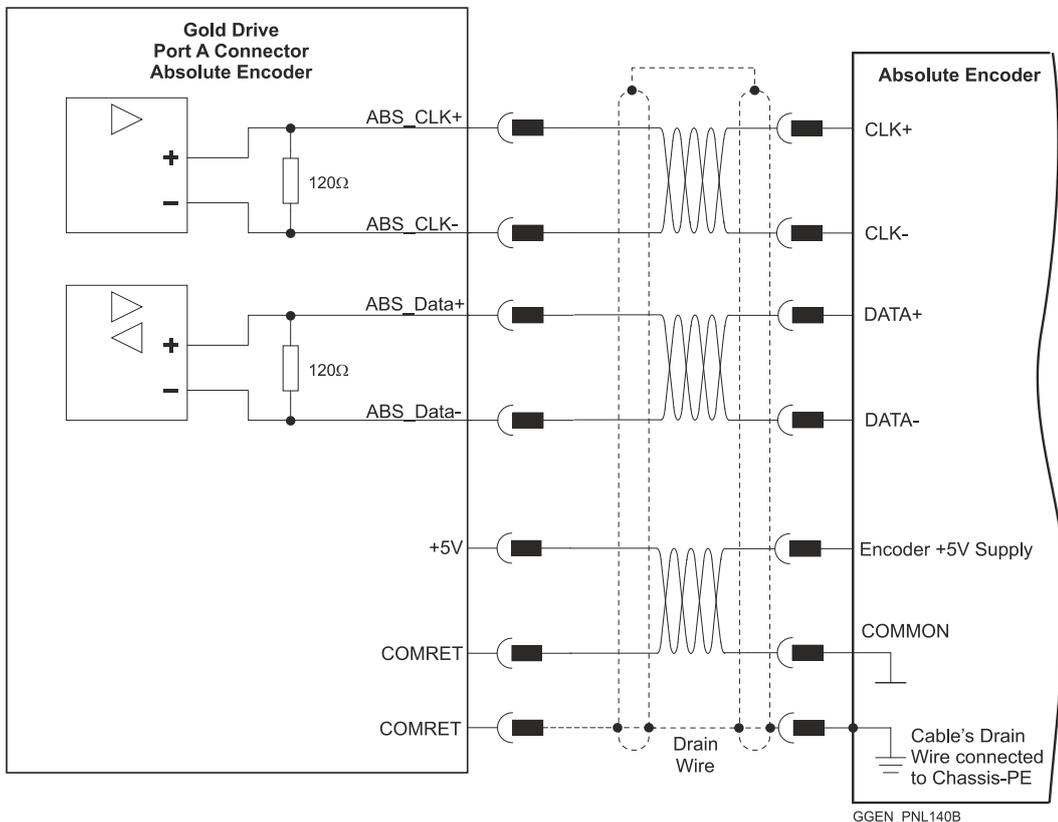
**Figure 23: Absolute Serial Encoder – Shrouded Type Connection Diagram Example**
