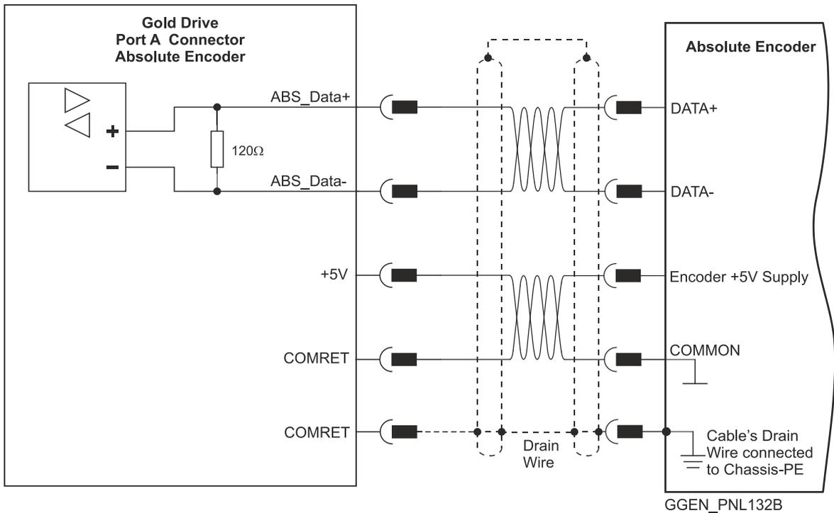
**Figure 25: Absolute Serial Encoder – Shrouded Type Connection Diagram Example for Sensors Supporting Data Line Only (NRZ types, e.g., Panasonic / Tamagawa / Sanyo / Nikon)**
