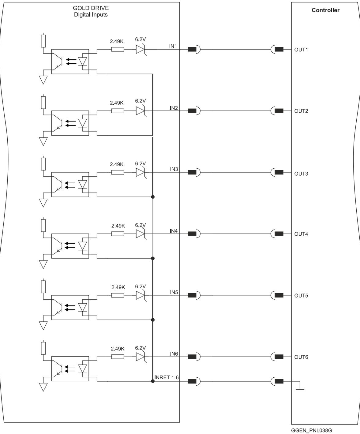
Figure 47: Digital Input Connection Diagram Example – Source PLC Option
