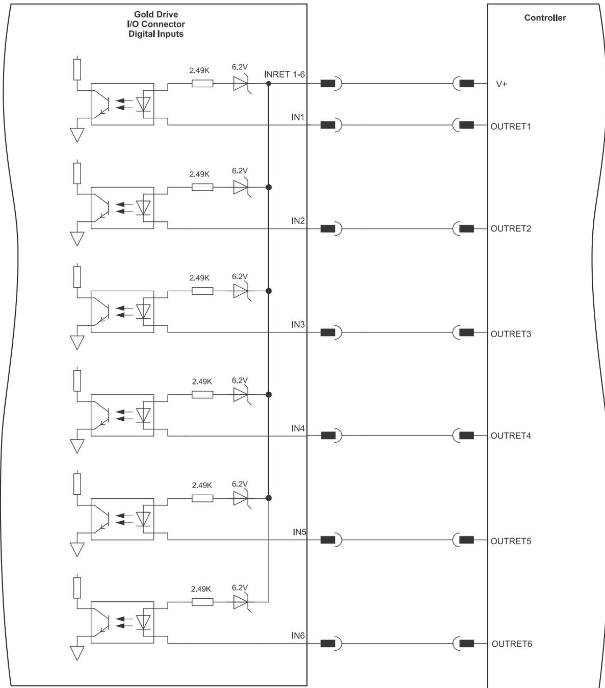
Figure 51: Digital Input Sink Mode Example – PLC voltage level Connection Diagram
