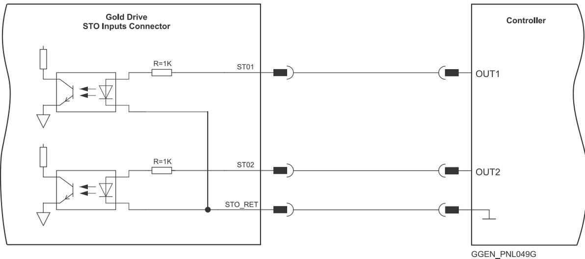
**Figure 10: STO Input Connection – TTL Option**
