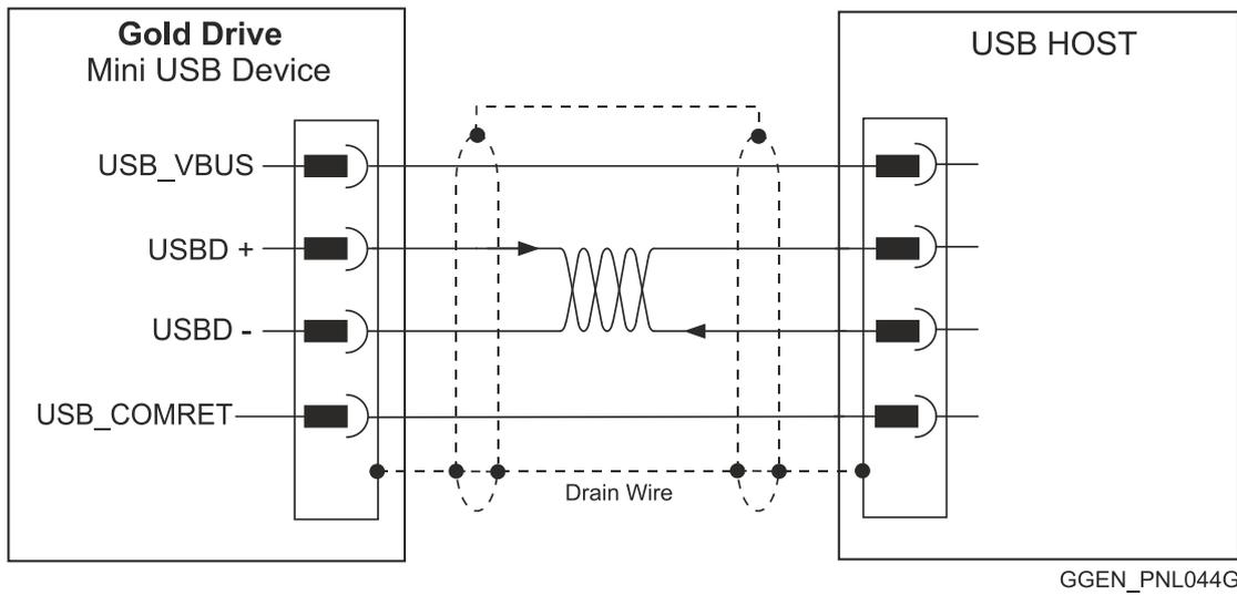
Figure 56: USB Network Diagram Example
