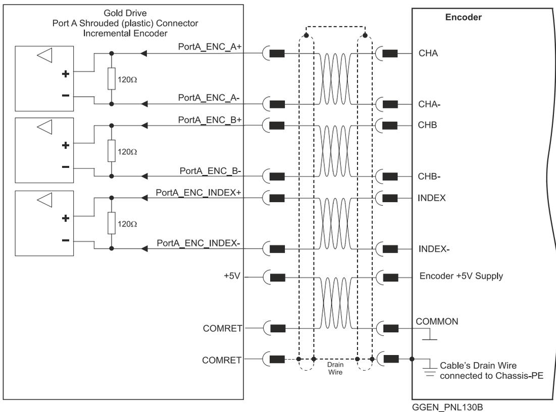
Figure 19: Port A Incremental Encoder Input – Shrouded Type Connection Diagram Example
