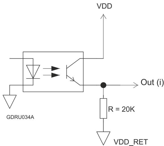
Figure 44: Digital Output TTL Schematic
