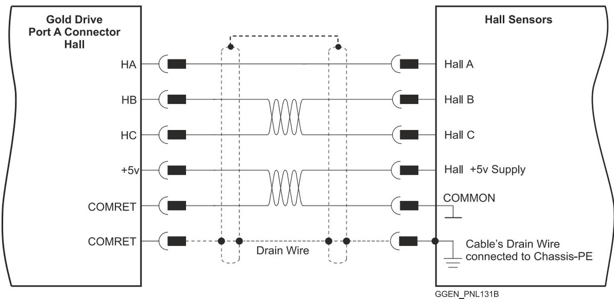
Figure 21: Hall Sensors Shrouded Type Connection Diagram Example
