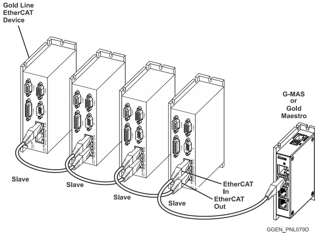
Figure 61: EtherCAT Network with No Redundancy
