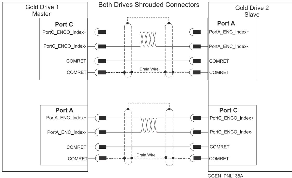
Figure 39: Port C to Port A Shrouded Type Connections Example
