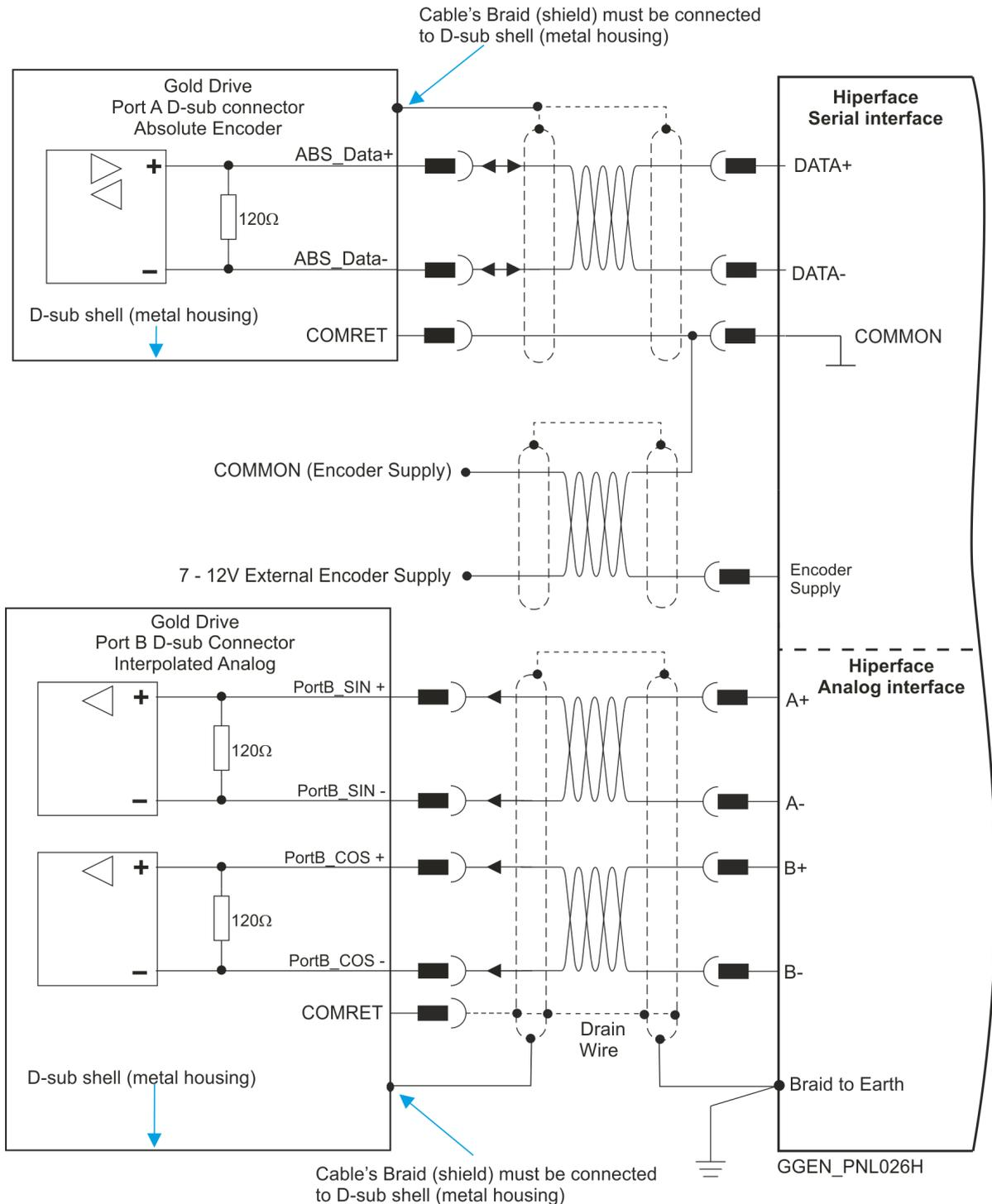
Figure 26: Absolute Serial Encoder – D-Type Connection Diagram Example for Stegmann Hiperface
