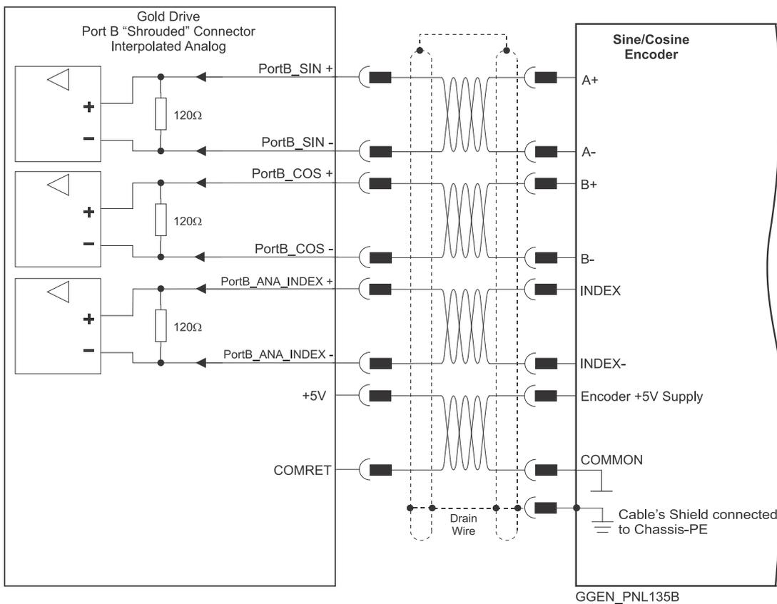
**Figure 32: Port B - Interpolated Analog Encoder Shrouded Type Connection Diagram Example**
