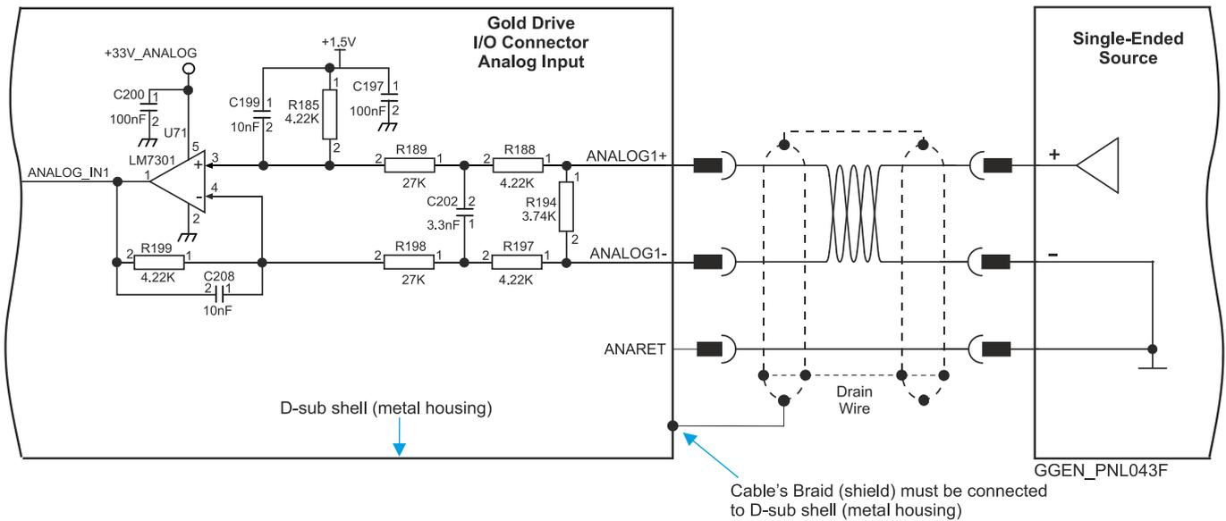
Figure 54: Differential Analog Input for D-Type connector
