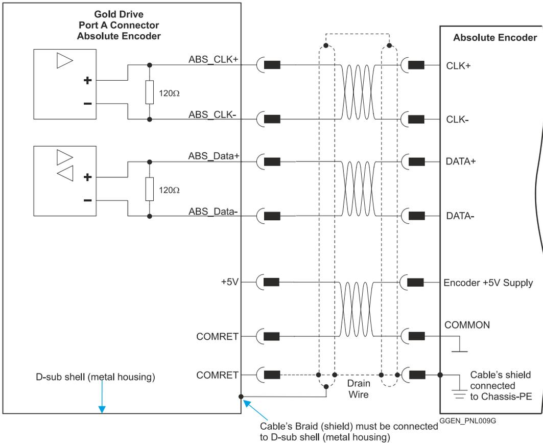
**Figure 22: Absolute Serial Encoder – D-Type Connection Diagram Example**
