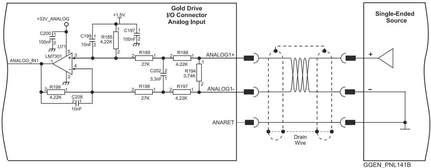
Figure 55: Differential Analog Input for Shrouded Type connector
