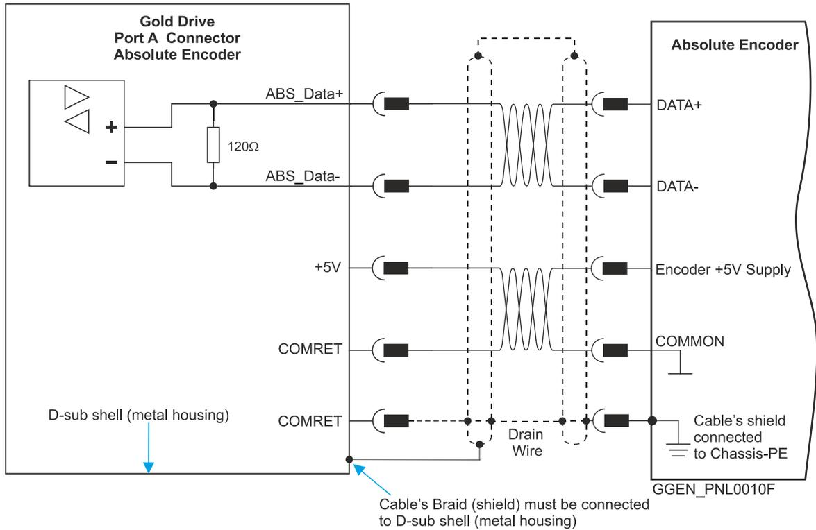
**Figure 24: Absolute Serial Encoder – D-Type Connection Diagram Example for Sensors Supporting Data Line Only (NRZ types, e.g., Panasonic / Tamagawa / Sanyo / Nikon)**
