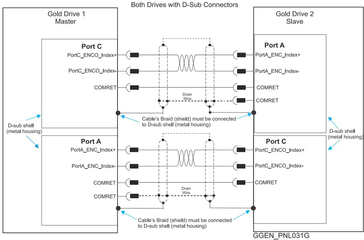
Figure 38: Port C to Port A D-Type Connections Example
