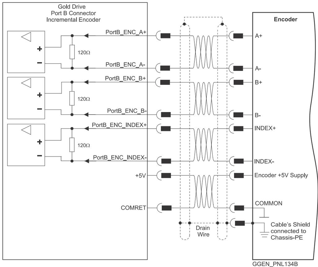
Figure 30: Port B Incremental Encoder Input – Shrouded Type Connection Diagram Example
