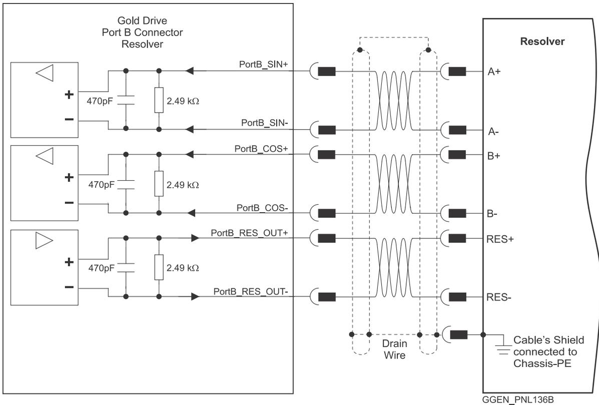
Figure 34: Port B – Resolver Shrouded Type Connection Diagram Example
