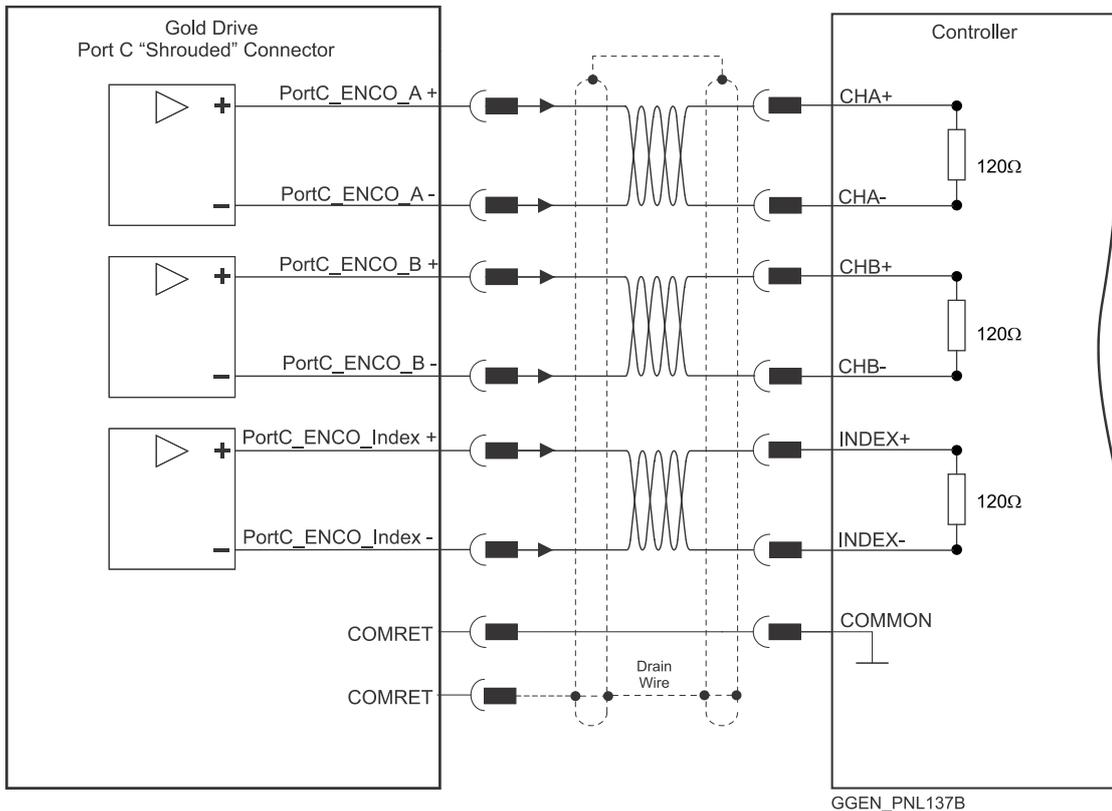
Figure 36: Encoder Differential Output – Shrouded Type Connection Diagram Example
