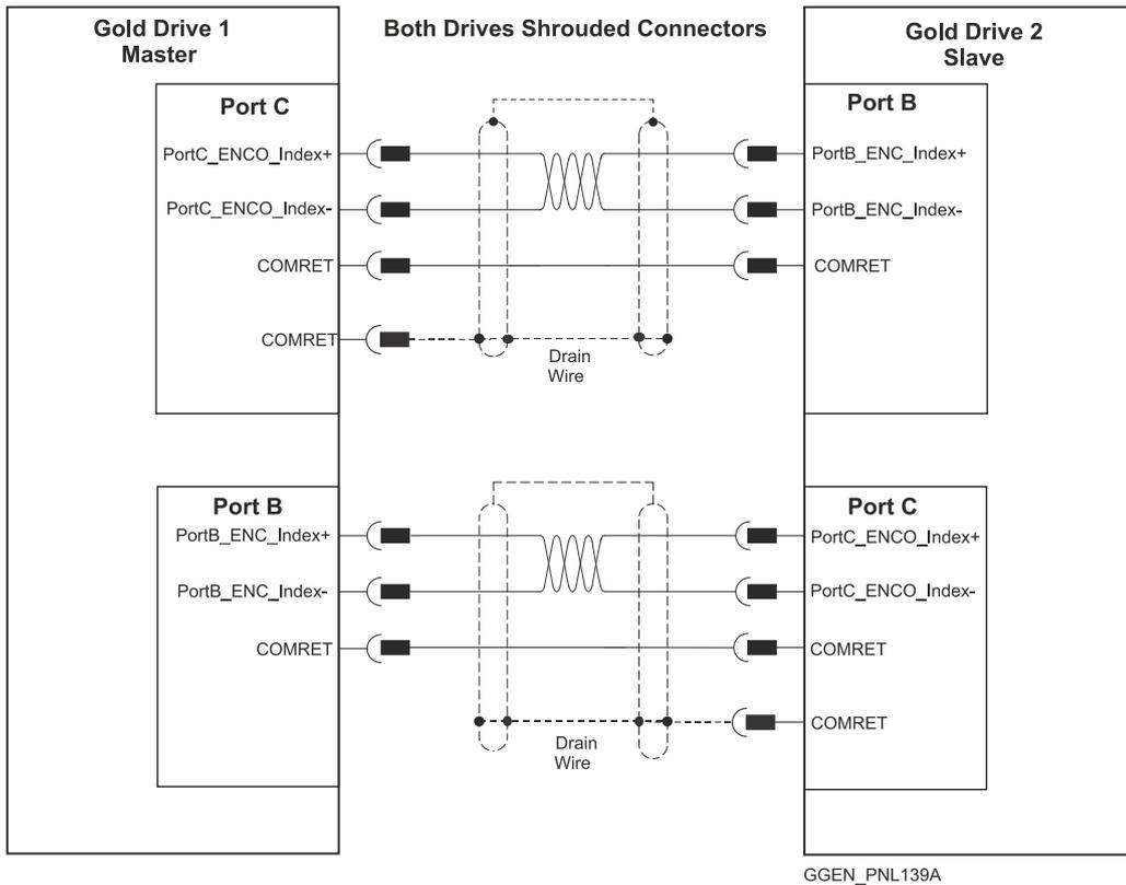
Figure 41: Port C to Port B Shrouded Type Connections
