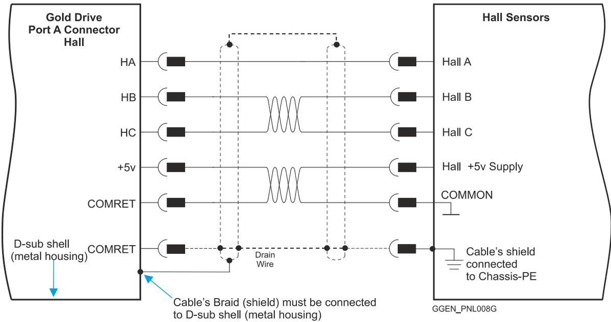
Figure 20: Hall Sensors D-Type Connection Diagram Example
