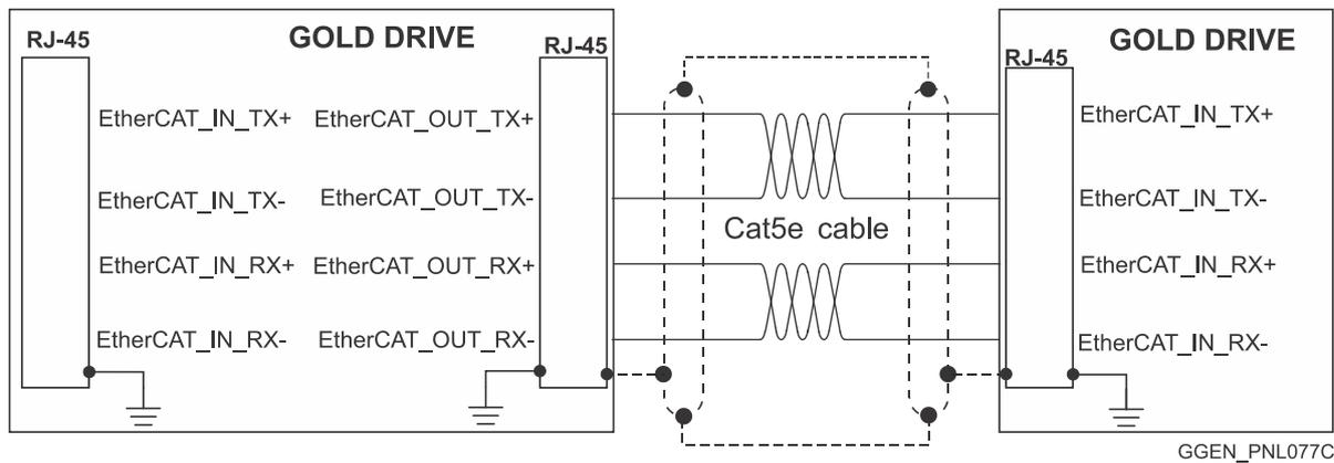
**Figure 57: EtherCAT RJ-45 Connections Example**
