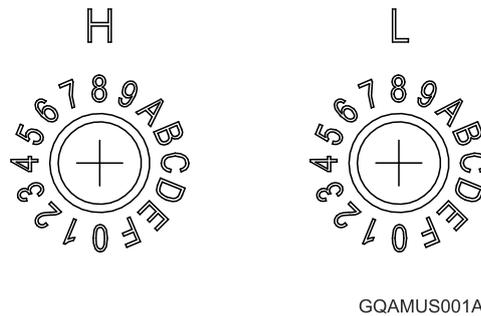
Figure 60: EtherCAT Address Switches
