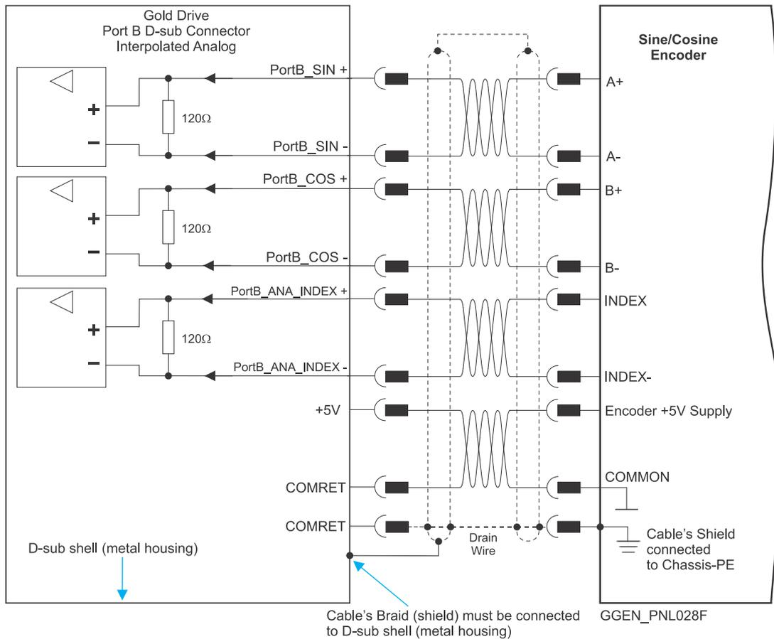
**Figure 31: Port B - Interpolated Analog Encoder D-Type Connection Diagram Example**
