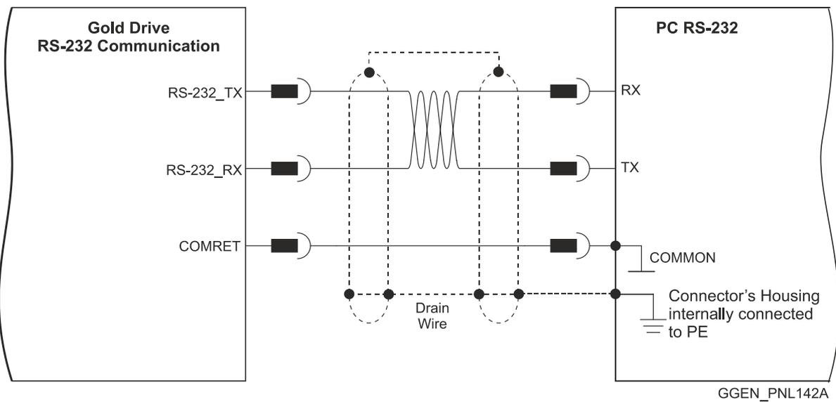
Figure 65: RS-232 RJ-45 Connection Diagram Example
