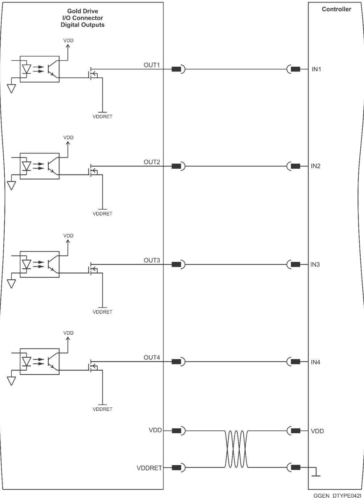
**Figure 53: Digital Output Example as Sink Configuration Connection Diagram**
