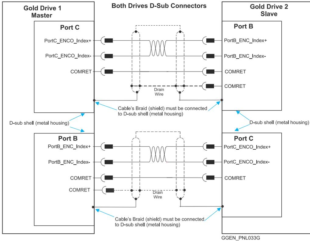
Figure 40: Port C to Port B D-Type Connections
