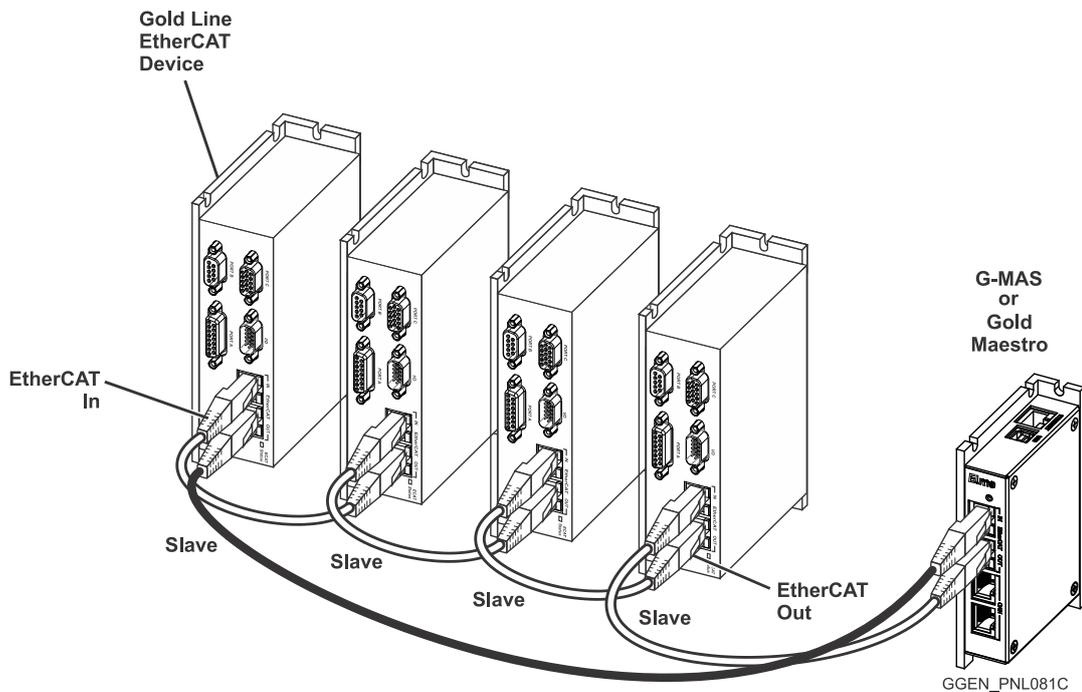
Figure 62: EtherCAT Network with Redundancy
