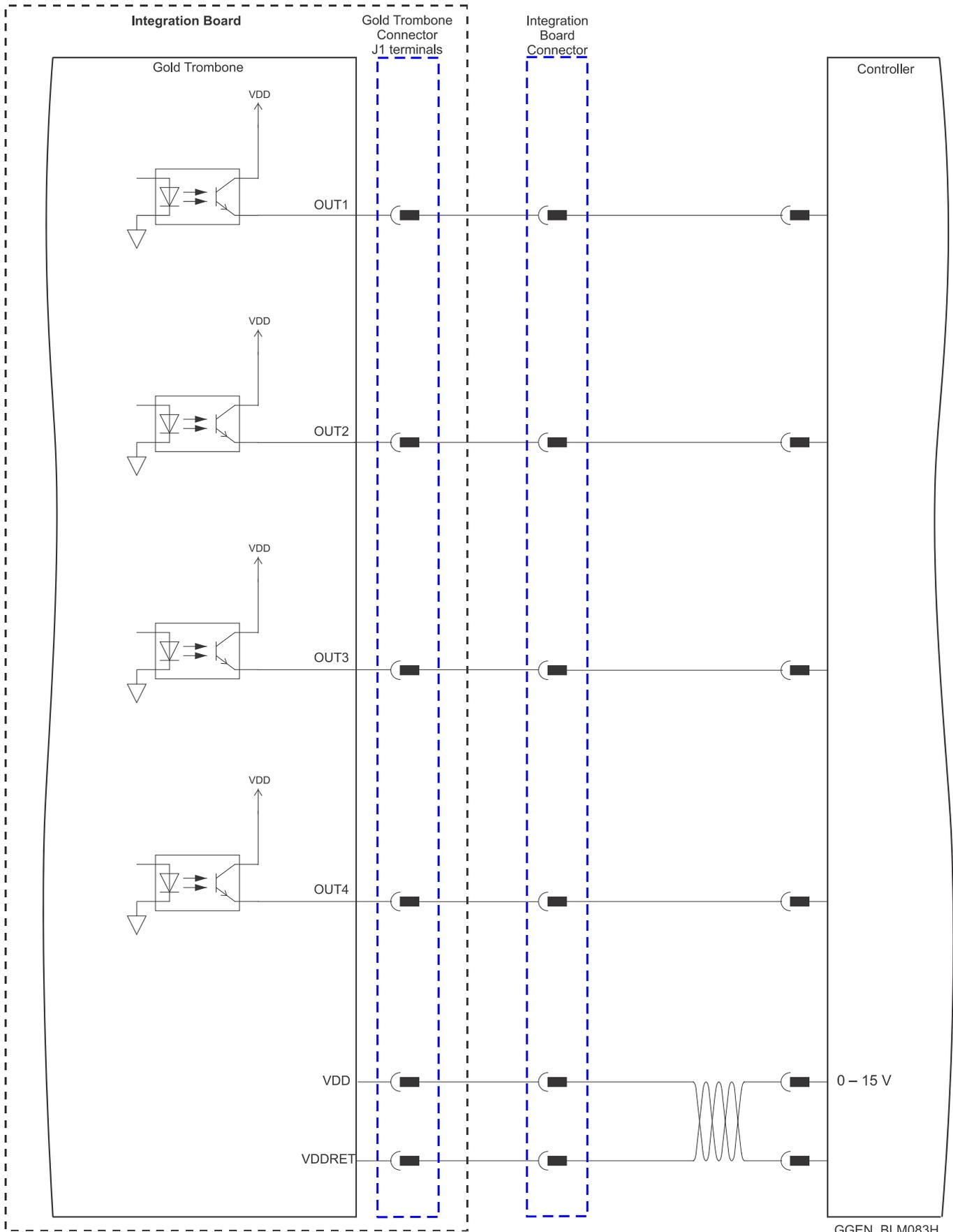
Figure 49: Digital Output Connection Diagram
