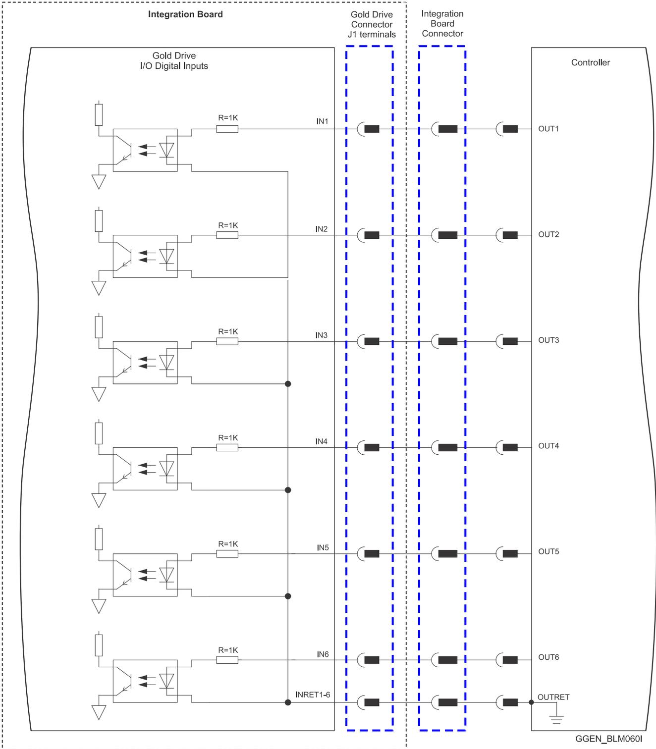
Figure 45: Digital Input TTL Mode Connection Diagram
