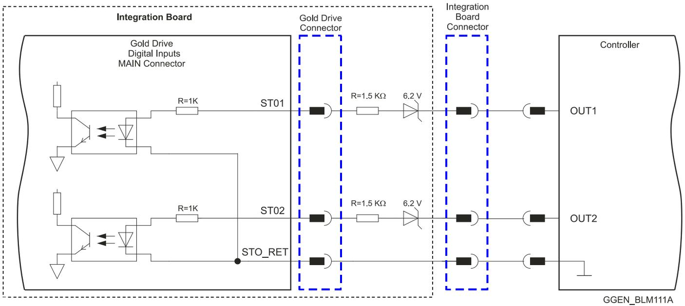
Figure 18: STO Input Connection – PLC Source Option for the G-WHI, G-BEL, G-GUT, and G-TWI
