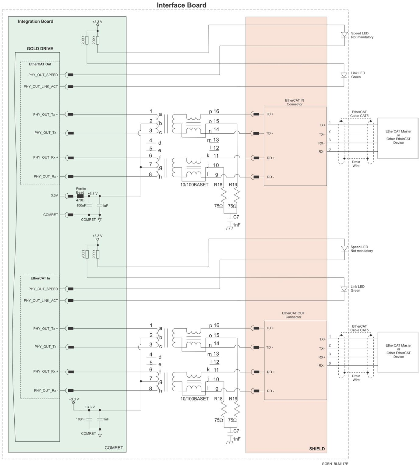
Figure 58: EtherCAT Connection Schematic without Magnetic Diagram
