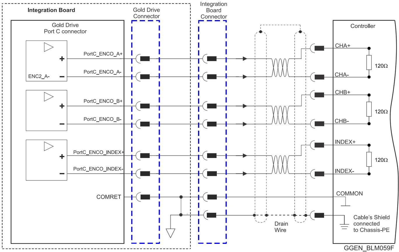
Figure 36: Emulated Encoder Differential Output – Recommended Connection Diagram
