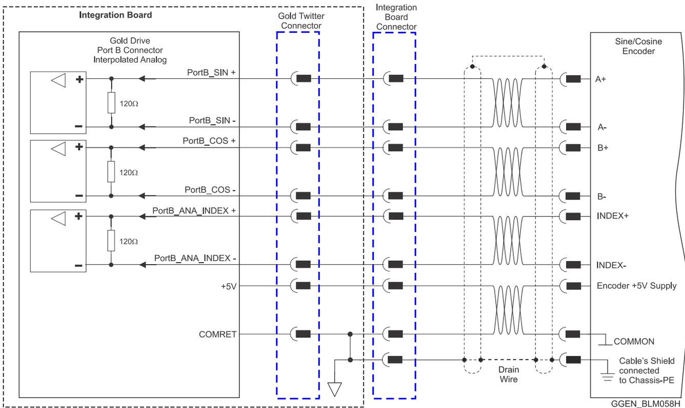
Figure 34: Port B - Interpolated Analog Encoder Connection Diagram
