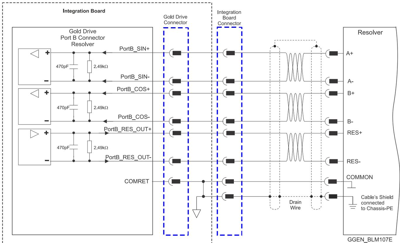
Figure 35: Port B – Resolver Connection Diagram
