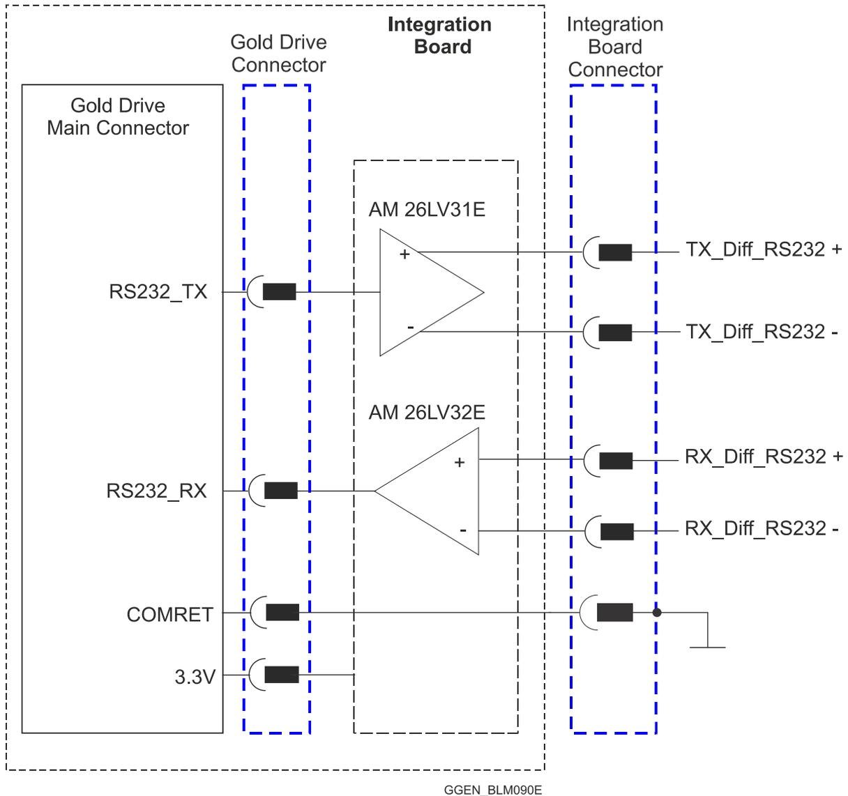
Figure 65: Differential RS232 Interfacing
