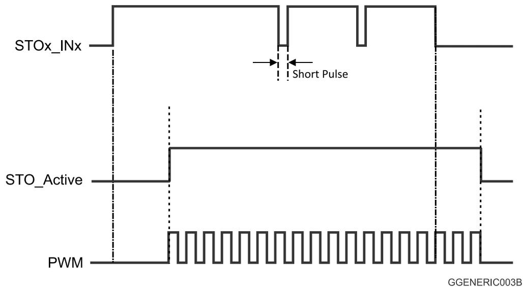
Figure 13: Timing Diagram of short pulses
