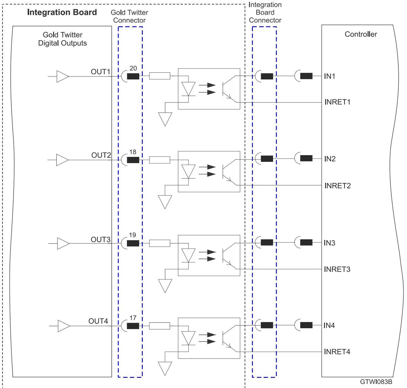
Figure 53: Digital Output 5V and 3.3V Level Mode Connection Diagram
