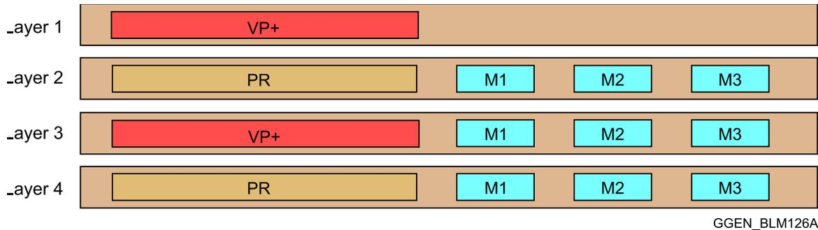
Figure 7: Power conductor split between several planes
