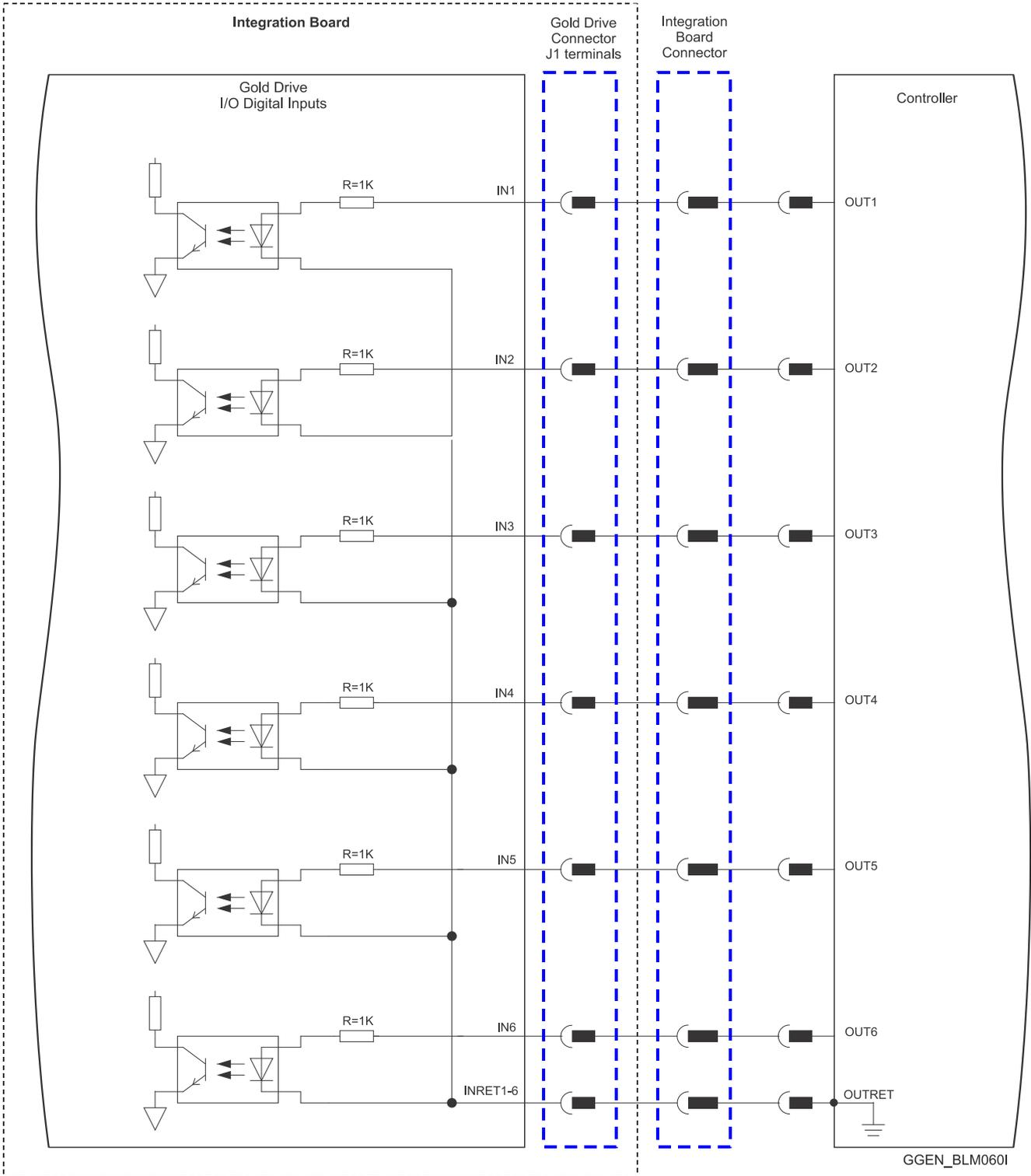
Figure 41: Digital Input TTL Mode Connection Diagram
