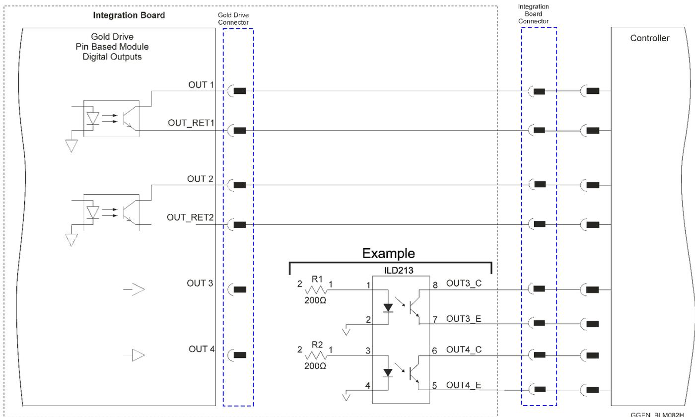
Figure 43: Digital Output Connection Diagram – TTL Connection
