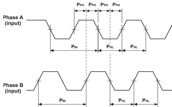
Figure 32: Main Feedback - Encoder Phase Diagram
