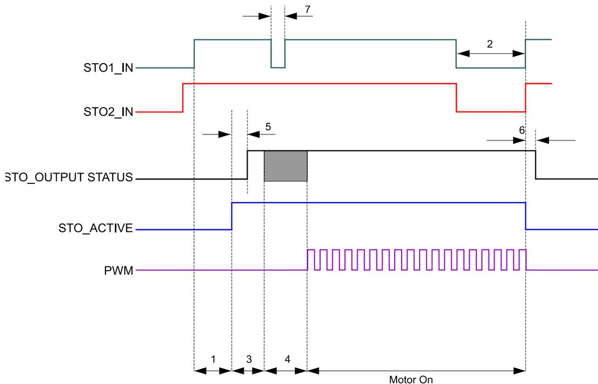
Figure 23: STO Timing Diagram
