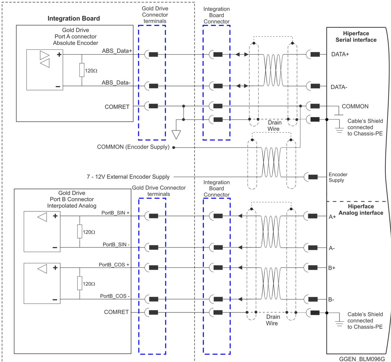
Figure 31: Absolute Serial Encoder – Recommended Connection Diagram for Stegmann Hiperface
