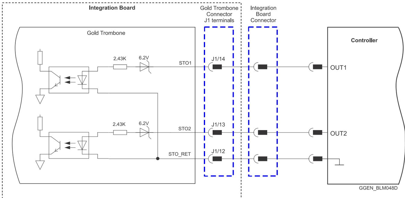
**Figure 17: STO Input Connection – PLC Source Option for the G-TRO**
