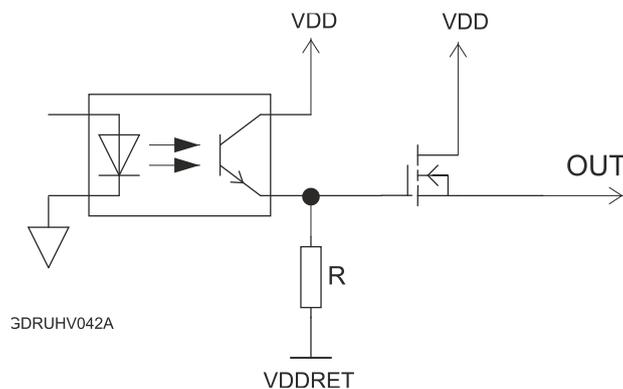
Figure 50: Digital Output Schematic – Source Mode PLC Level
